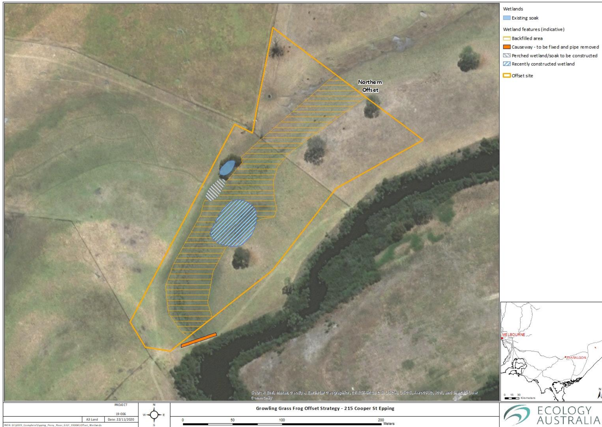
Figure 8 Indicative location of the existing soak, new wetland, proposed perched wetland and the causeway at the northern offset site
